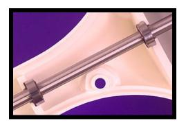
Seating of bearings into housing. Note that the bearings are positioned against their retaining clips, and on the inside of the plastic wall.
