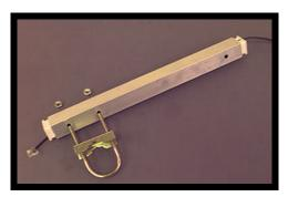
Aluminum tube assembly. Holes must be drilled in the aluminum tube for the mounting clamp and housing fastener. A Radio Shack type 15-826 or equivalent U clamp may be used. Note the placement of the end cap notches and cable
