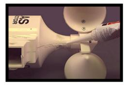
Sealing the housing. A clear sealant such as GE's RTV-118 or equivalent should be applied to the seams of the weather station housing as shown. Take care not to affect the free movement of the wind cup assembly. An excess of sealant is shown here for illustration purposes, but only the minimum amount required to waterproof the seams is needed
