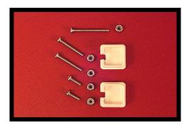
Hardware supplied with the weather station kit. The two pairs of screws and locknuts fasten the housing together. The single long screw and locknut fasten the square aluminum tube to the housing. Cut or file notches in the two plastic end caps similar to those shown above for the wire to enter and exit the tube.
