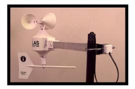
Mounting the weather station. View from the mast showing arrangement of the "U" type mounting bracket and end cap. Notice that the cable comes out of the bottom side of the tube and forms a "drip loop." For purposes of clarity, the end cap is shown only partially inserted in the tube, but should be fully seated in the tube
