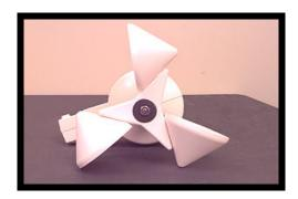
**View from the top** of the wind speed assembly, showing 1" diameter washer and nut in place
