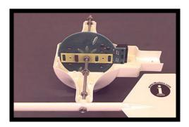
View from the bottom of housing, showing component side of PCB facing wind direction rotor frame assembly. Notice that the wind direction rotor has a single magnet and is aligned parallel to the wind vane.
